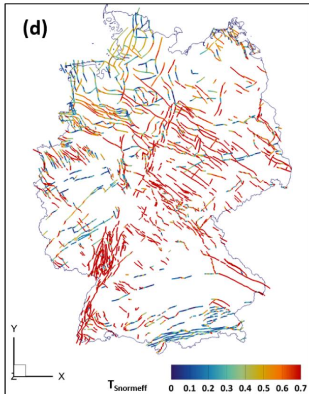
Slip tendency of major vertical faults in onshore Germany (Röckel et al., 2022)
